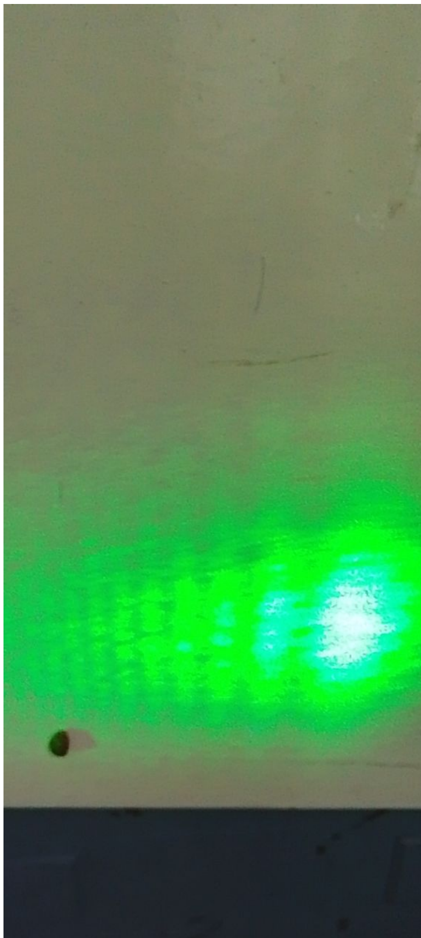
Figure 5: Diffraction pattern with a flux cross-section close to the appearance of general background illumination. The position of the maximum relative to the marker remains unchanged.
